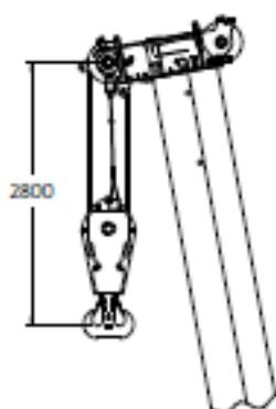
Dimension shown is for the largest Genie furnished hookblock with anti-tie block attached.
