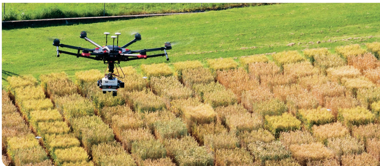
Unmanned aerial vehicle carrying colour and thermography cameras to assess height and temperature of wheat breeding plots (photo Norbert Kirchgessner, ETH Zurich)
