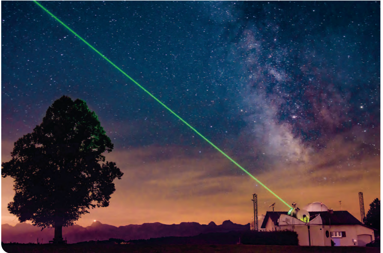
Figure 17: Laser beam transmitted from the 1-metre ZIMLAT telescope to measure the distances of artificial satellites with a mm-accuracy. (Image: Emiliano Cordelli [AIUB])
