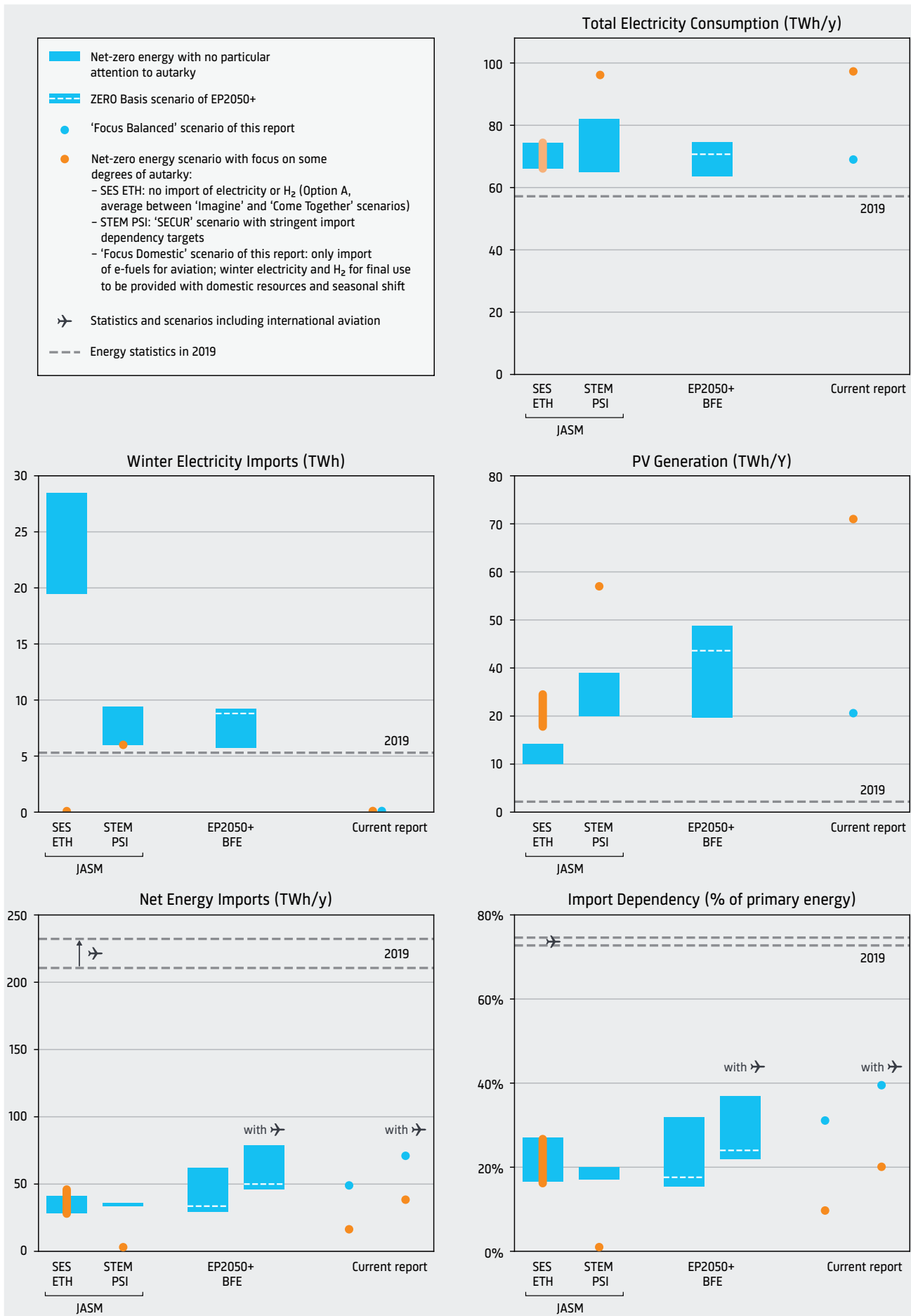
Fig. 9. Key 'performance parameters' of the Swiss energy system in 2050 according to estimates from various studies and scenarios: total electricity consumption, winter electricity imports, PV generation, net energy imports and import dependency (ratio of net energy imports to the gross (primary) energy supply).
