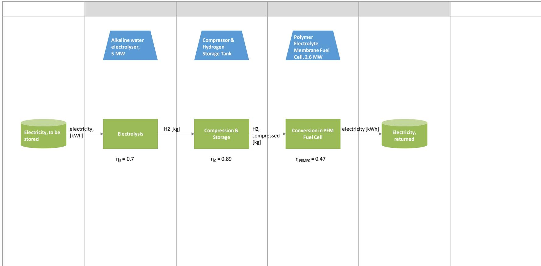
Figure 19: Representation of the power-to-hydrogen-to-power storage system.
