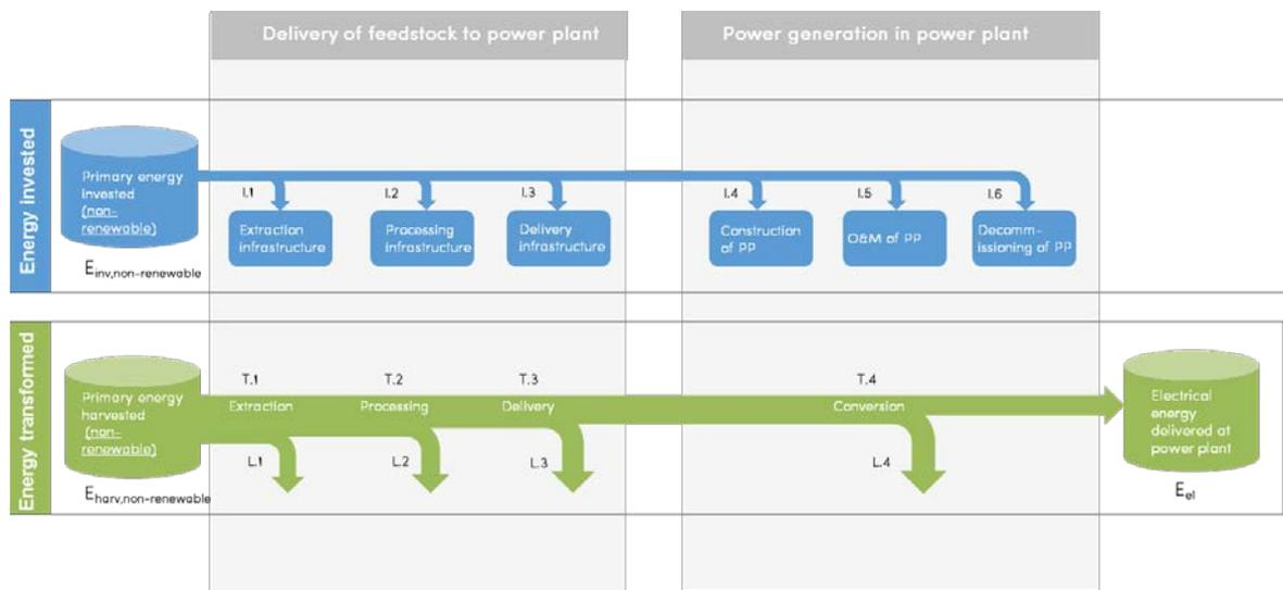
Figure 4: Energy flows for calculation of the nr-CED for a fuel based power generation system.
