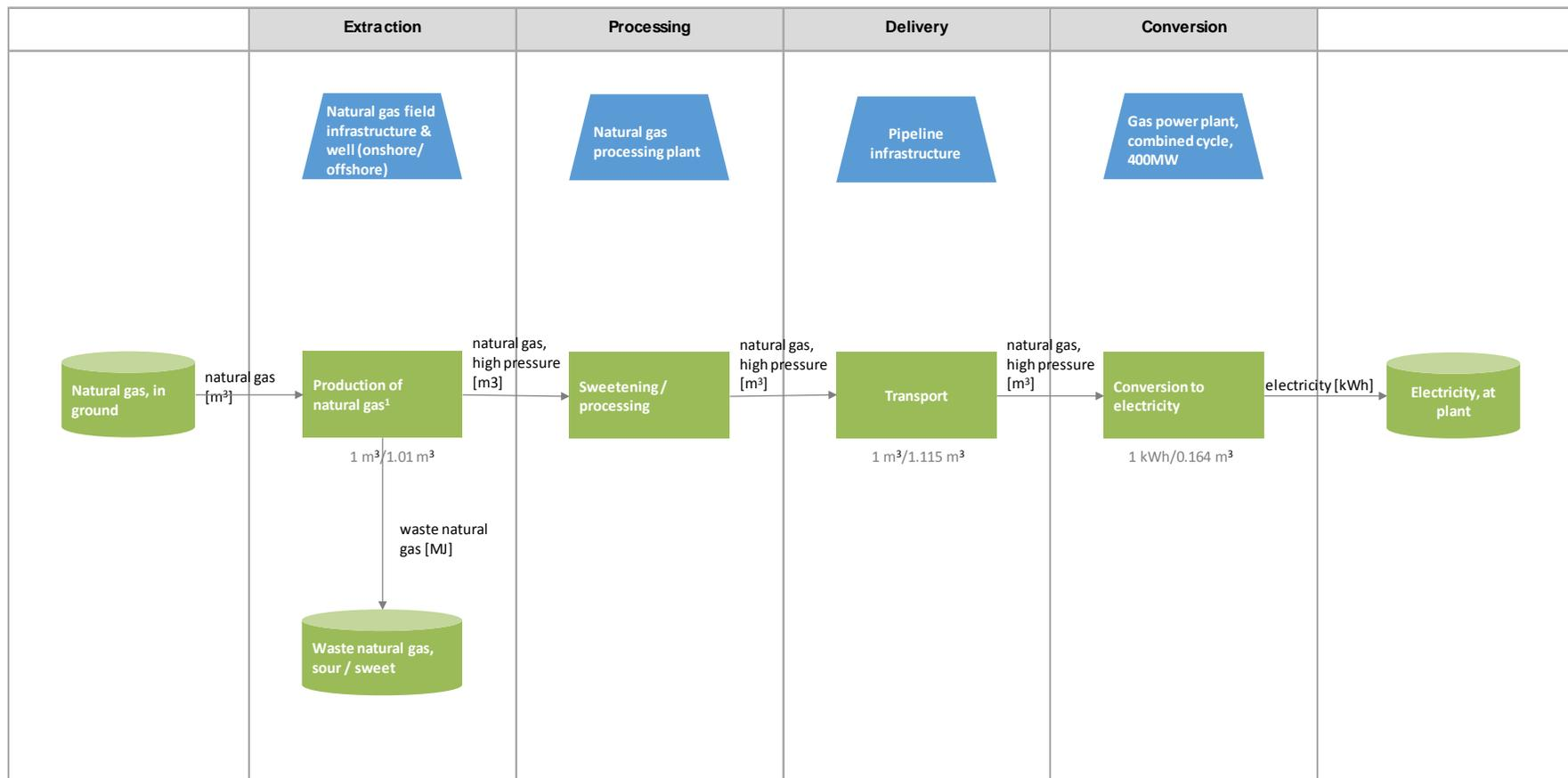
**Figure 8: Representation of the natural gas (CCGT) based power generation system in ecoinvent.**
