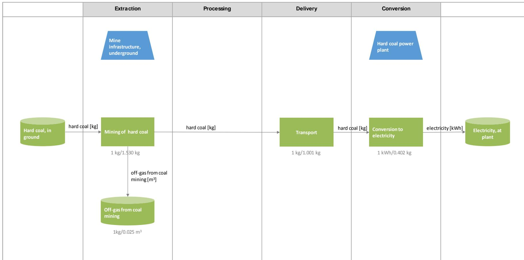
**Figure 7: Representation of the hard coal based power generation system in ecoinvent.**
