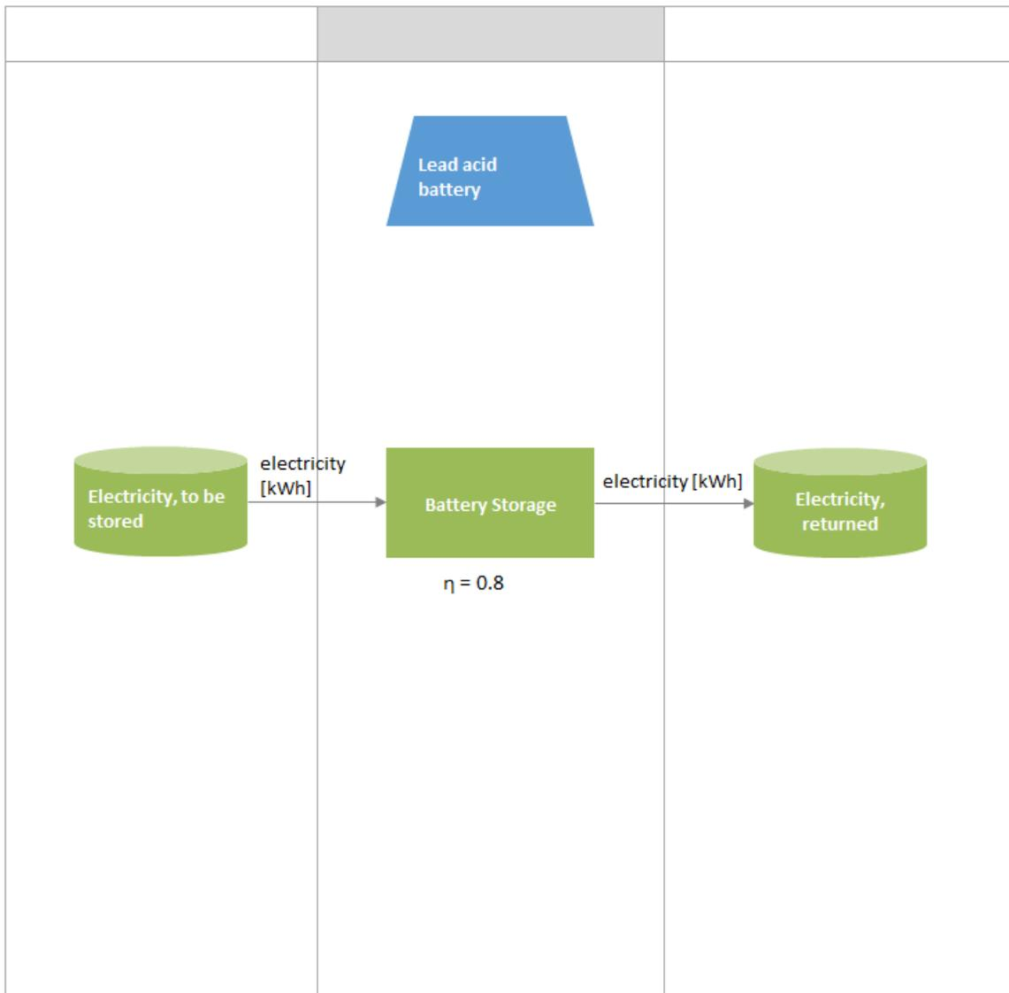
Figure 16: Representation of the lead acid battery storage system.
