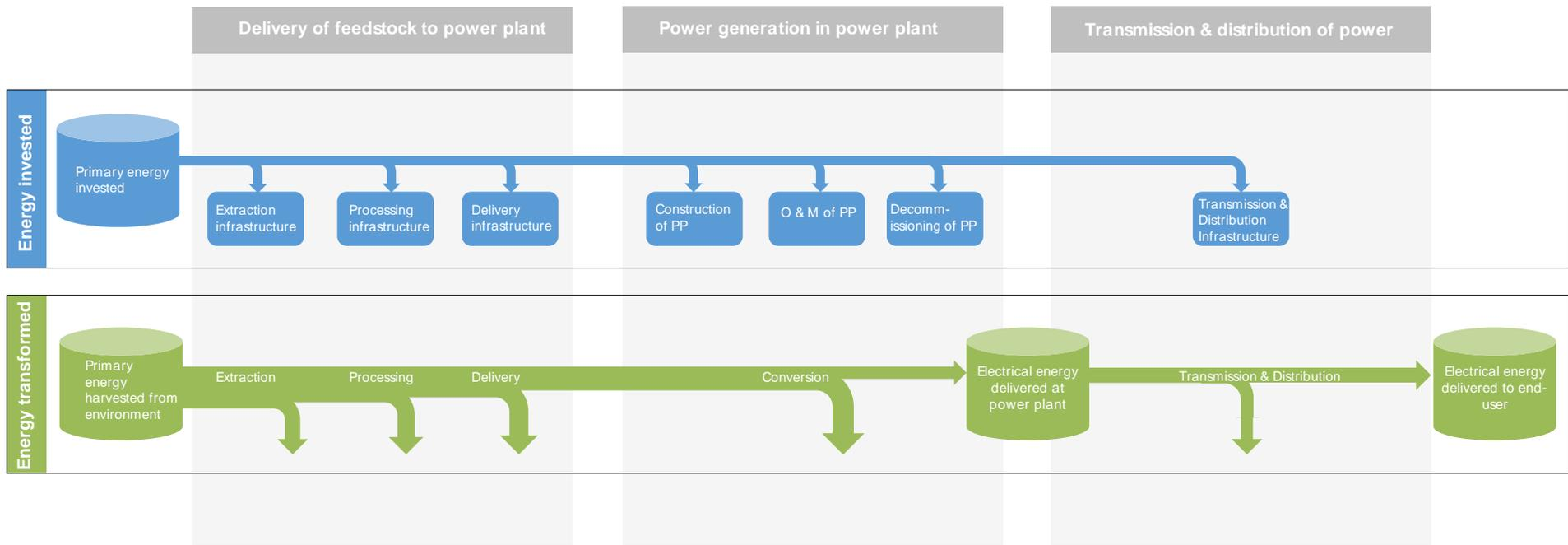
Figure 2: Extended energy flows of fuel based power generation system including transmission and distribution.
