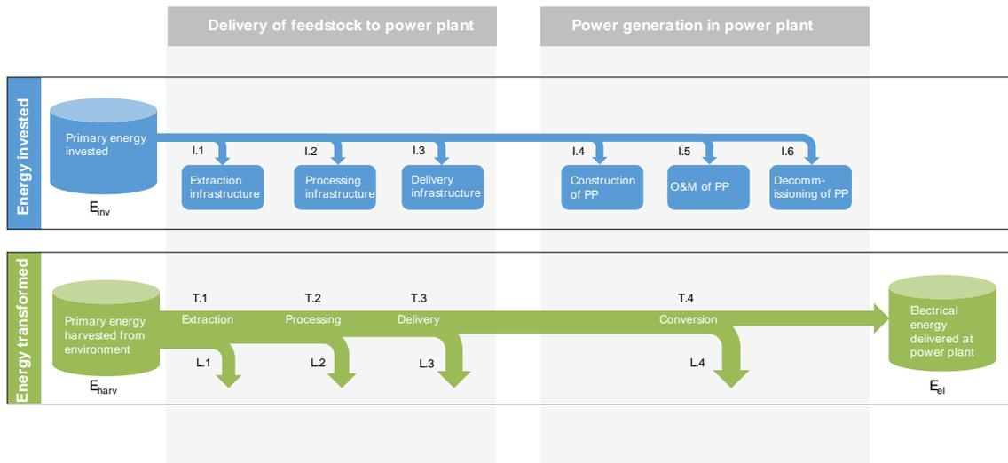
Figure 5: Energy flows for calculation of the EROI for a fuel based power generation system.
