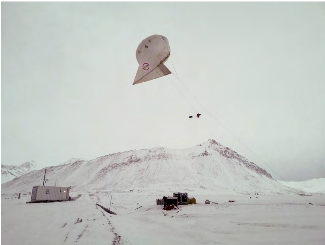
Figure 1.4: HoloBalloon flying with the instrument platform hanging 12 m below the helikite. The container where aerosol measurements were performed is visible on the left. Photography taken by Jan Henneberger.
