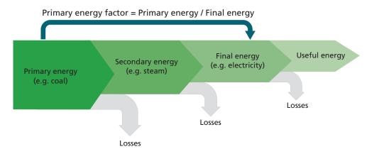
Figure 8 Losses occur at each stage in the process when fuels are converted to useful energy (Hirzel et al. 2023).
