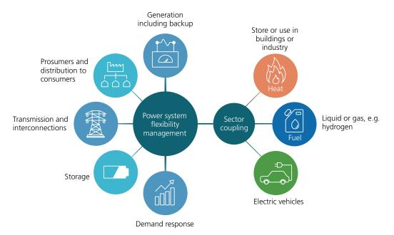
Figure 12 Flexibility management measures for electricity grids include demand response, storage, interconnections, and backup generation, together with sector coupling (adapted by EASAC, on the basis of IRENA 2024a).
