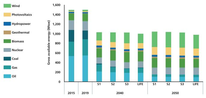
Figure 6 EU gross available energy<sup>2</sup> scenarios (S1, S2, S3, and LIFE) were used in the PRIMES modelling for the impact assessment of EU 2040 targets (EC 2024a). Note: 1 million tonnes of oil equivalent (Mtoe) = 11.63 terawatt-hours (TWh).
